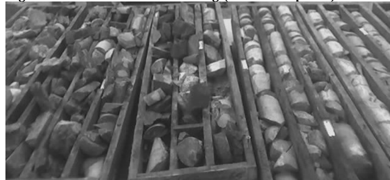
Figure 9: Half Core After Cutting (left side of photo)
